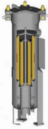
Coalescer and separator mounted in the RVFS housing. Fluid/fuel is passed from the outside of the coalescer to the inside. The coalescer element provides primary filtration of the fuel as well as coalescing free water from it. The clean fuel passes through the separator barrier and into the outlet of the housing. The coalesced water droplets are repelled by the hydrophobic barrier and are collected in the sump of the housing. The sump should be drained routinely.
