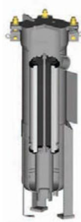
Mounting shown – Parker's patented FS synthetic microfilter series. The microfilter features a water resistant, all synthetic media and provides 99.5% + efficiency at the stated 1, 5, 10 & 25 micron ratings.
